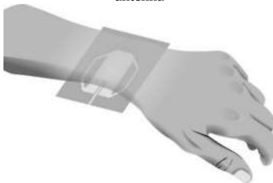
Fig. 7. Proposed antenna placement for measurement
