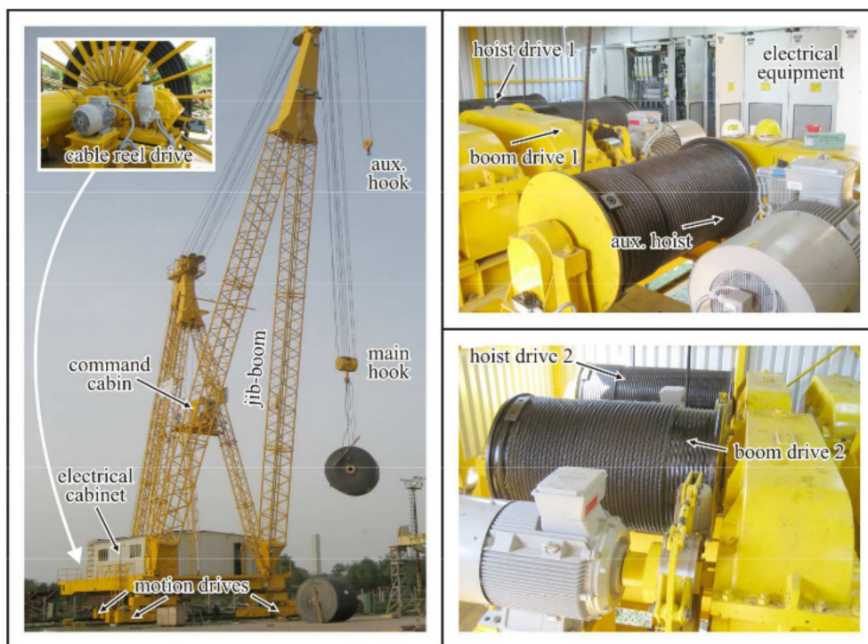
Fig. 13. Derrick crane with indicated drives.
