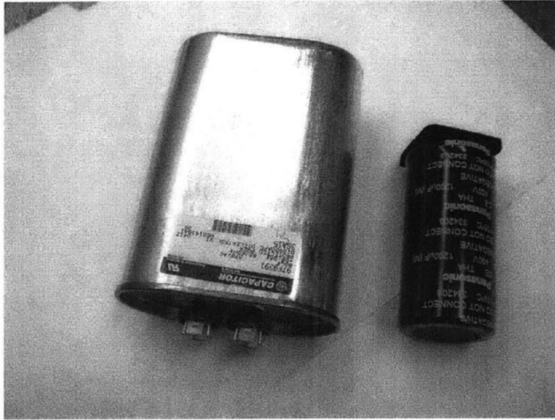
Figure 4.16: Comparison of 80 \mu\text{F} , 270 V AC and 1200 \mu\text{F} , 400 V DC capacitors
