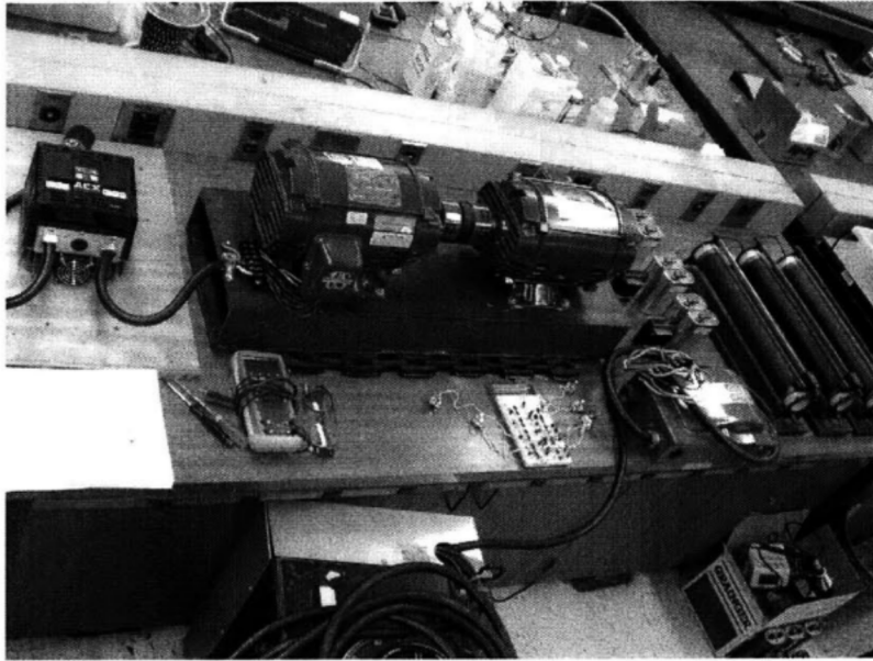
Figure 2.1: 2kW Test and Demonstration Platform
