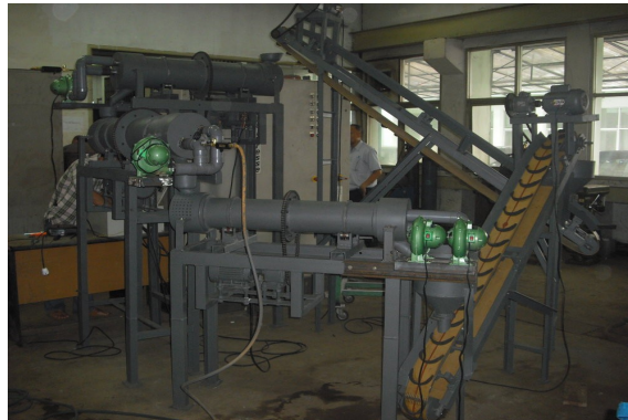
Figure 1 The Miniature of a Process Control Plant for Industrial Solid Materials
