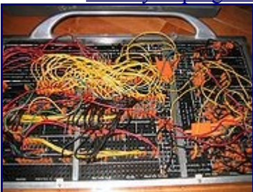
Wired plug board for an IBM 402 Accounting Machine .
