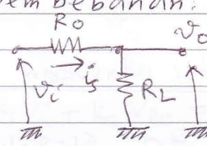
$$V_0 = \frac{R_L}{R_o + R_L} V_i$$
