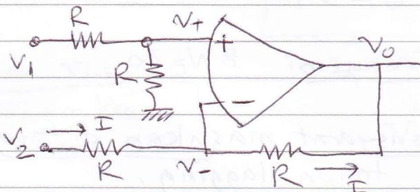
$$V_+ = \frac{R}{R+R} V_1 = \frac{1}{2} V_1$$
