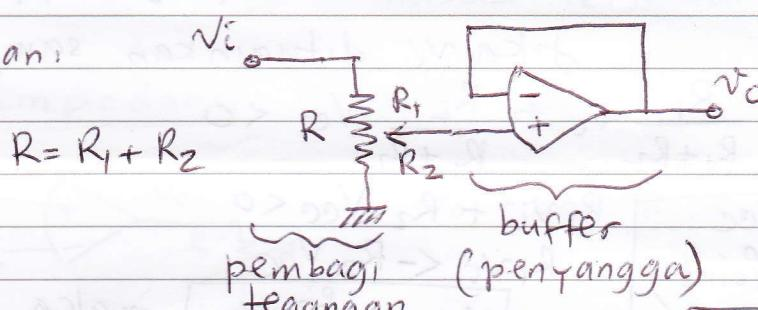
$$\begin{aligned} V_o &= V_- = V_+ \\ V_+ &= \frac{R_2}{R_1 + R_2} V_i \\ &= \frac{R_2}{R} V_i \end{aligned}$$
