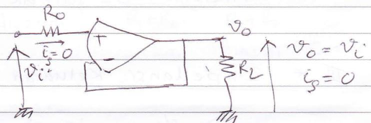
Sifat I  $\rightarrow V_0 = V_i = V_+ = V_-$
