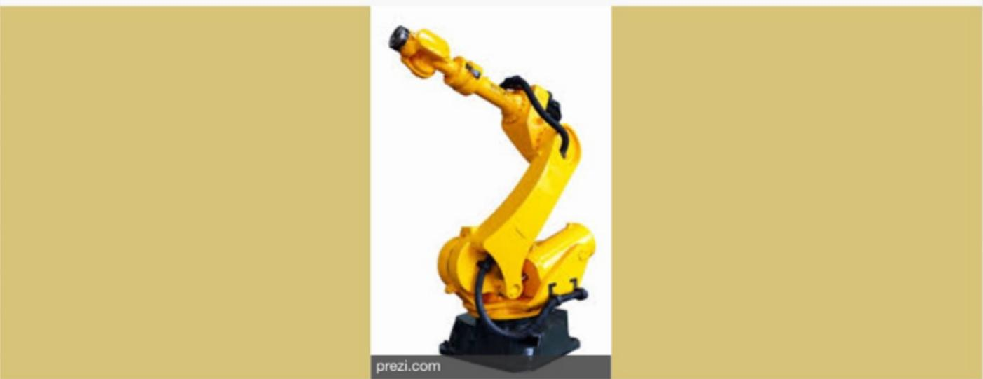
"Industrial robots. Industrial robot as defined by ISO 8373: An automatically controlled, reprogrammable, multipurpose manipulator programmable in three or more axes, which may be either fixed in place or mobile for use in **industrial** automation applications."
