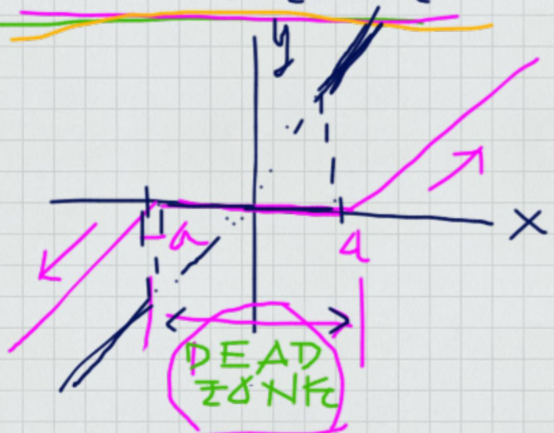
$$\begin{aligned} & |x(+)| \geq a \quad \text{supaya } y \neq 0 \\ & |x(+)| \leq a \quad y=0 \\ & -a \leq x(+) \leq a \end{aligned}$$
