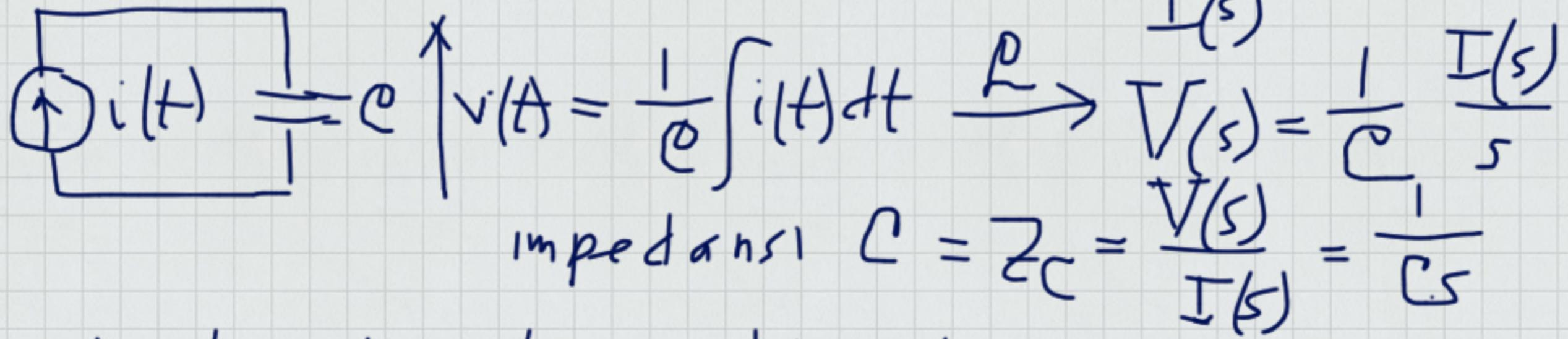
$$\text{Impedansi } C = Z_C = \frac{V(s)}{I(s)} = \frac{1}{C_s}$$
