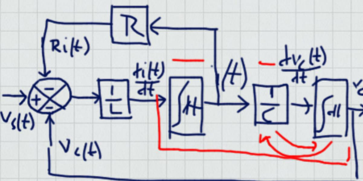
$$\begin{aligned} & * V_s(t) - V_c(t) = R i(t) + L \frac{di(t)}{dt} \quad (1) \\ & * i(t) = C \frac{dV_c(t)}{dt} \quad (2) \end{aligned}$$
