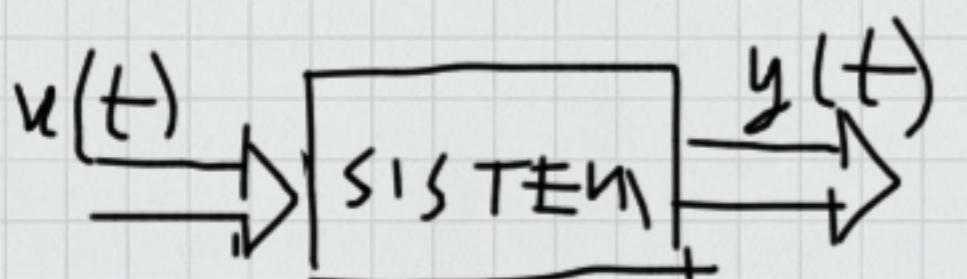
$$u(t) = \begin{bmatrix} u_1 \\ u_2 \\ \vdots \\ u_m \end{bmatrix} \quad [m \times 1]$$
