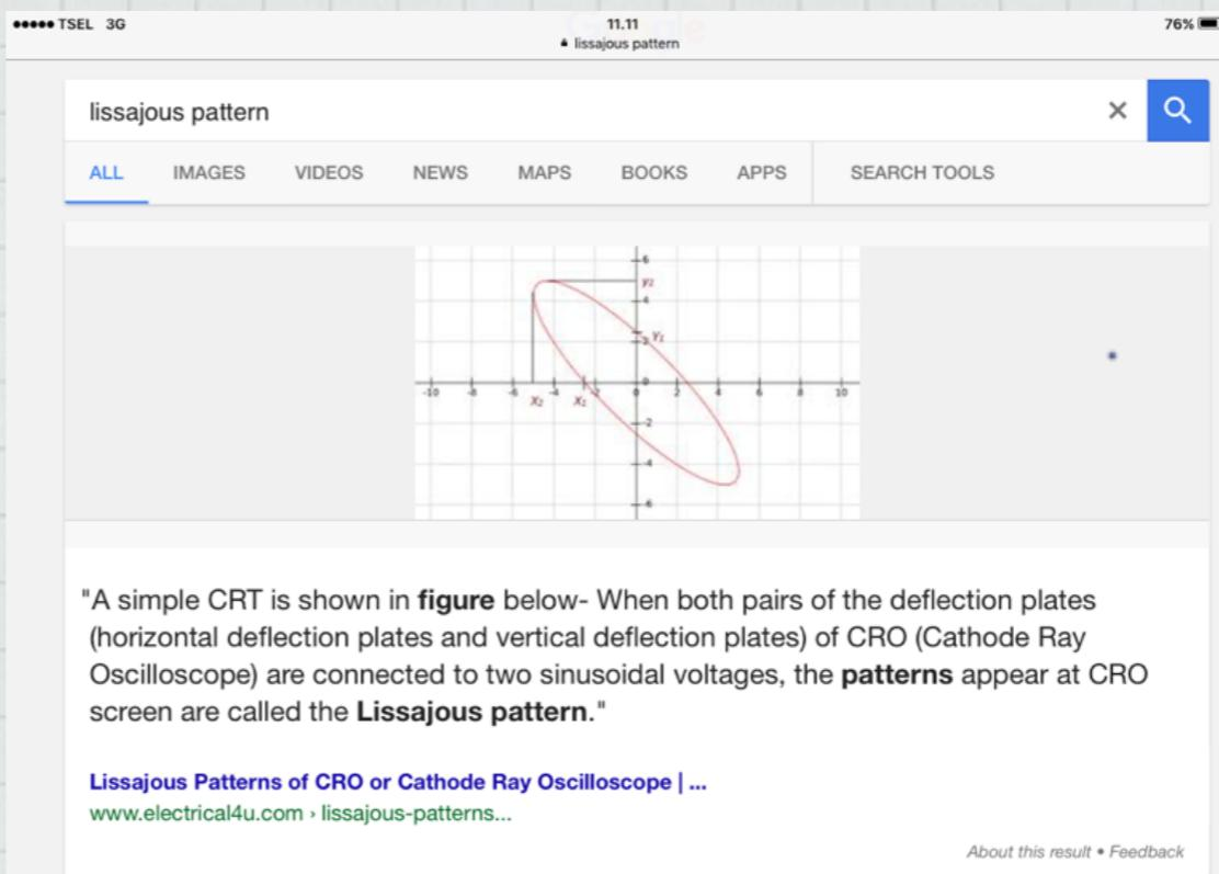
"A simple CRT is shown in figure below- When both pairs of the deflection plates (horizontal deflection plates and vertical deflection plates) of CRO (Cathode Ray Oscilloscope) are connected to two sinusoidal voltages, the patterns appear at CRO screen are called the **Lissajous pattern**."
