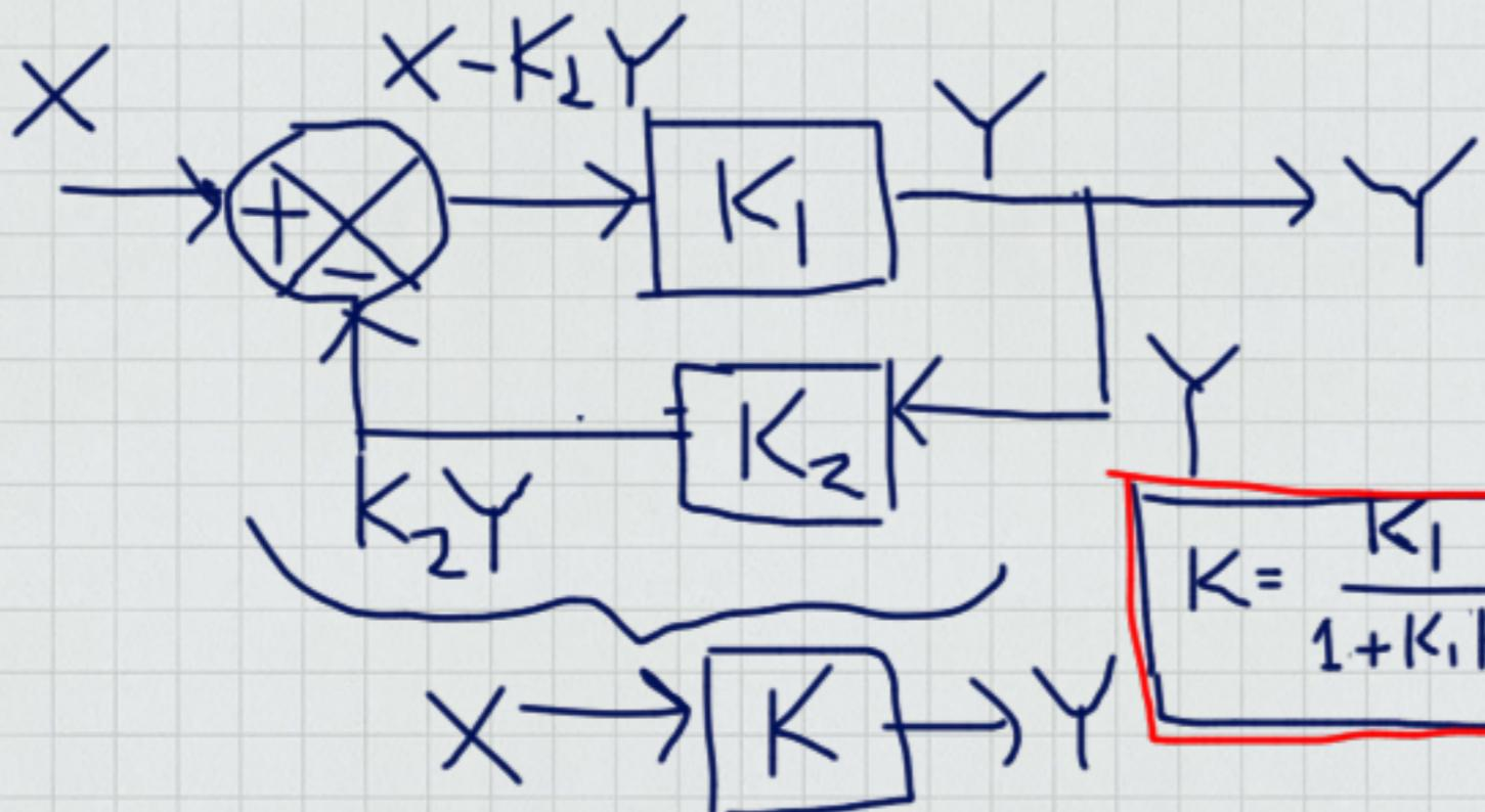
$$\begin{aligned} Y &= K_1(X - K_2Y) \\ &= K_1X - K_1K_2Y \\ Y + K_1K_2Y &= K_1X \\ (1 + K_1K_2)Y &= K_1X \\ Y &= \left( \frac{K_1}{1 + K_1K_2} \right) X \end{aligned}$$
