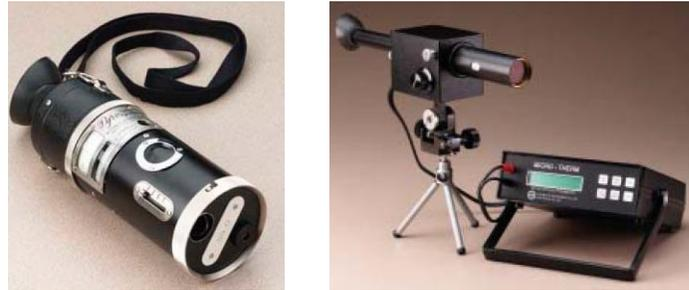
Gambar 3.84. Optical Pyrometer
