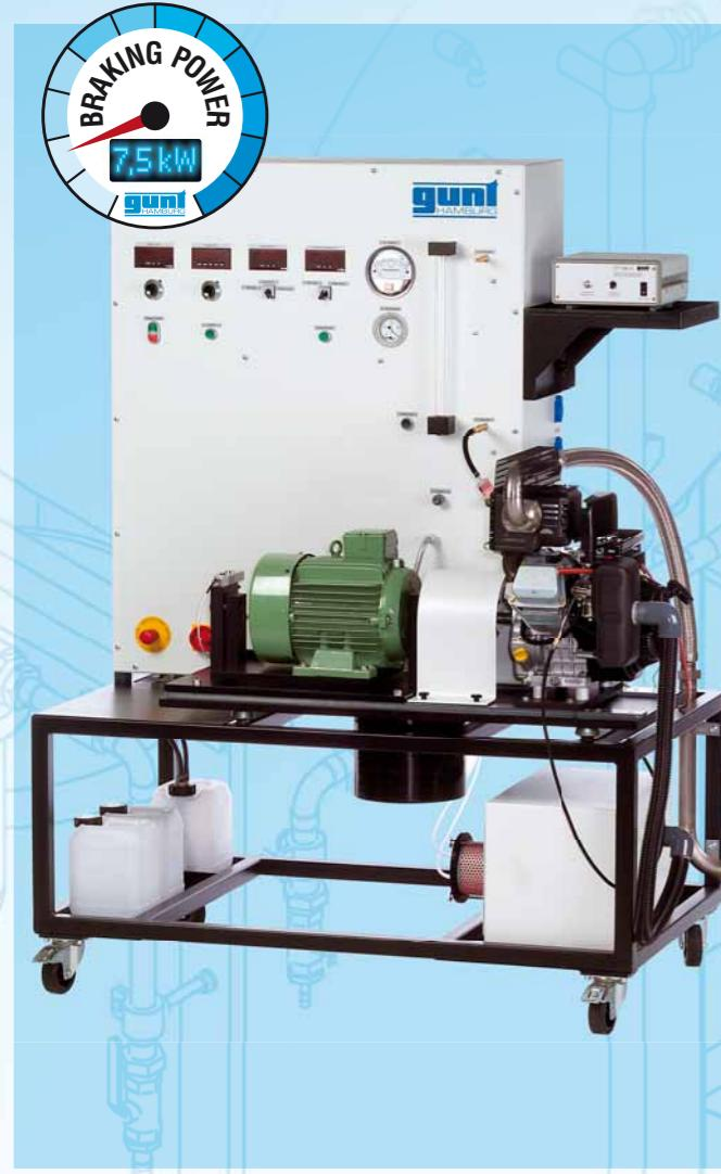
The CT 110 test stand can be used for a wide range of experiments on small internal combustion engines with a power output of up to 7.5 kW. There is a choice of 4 different engines, which can be mounted on the base plate in the test stand as required. A test engine can be installed in just a few minutes.
