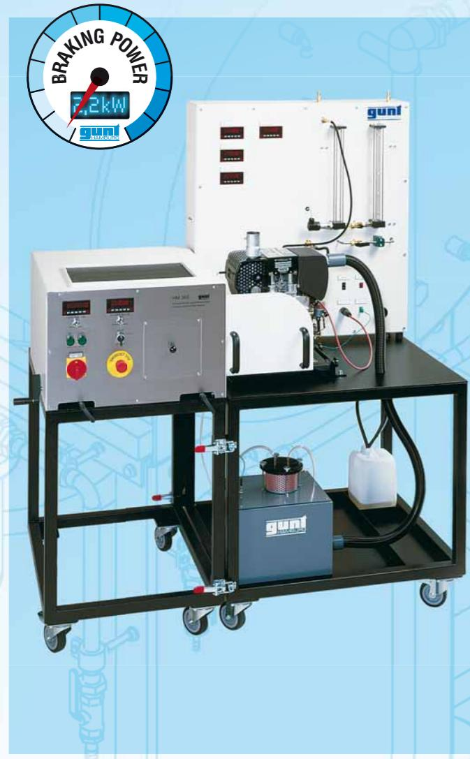
In conjunction with the HM 365 Universal brake and drive unit, the CT 159 can be used for a wide range of experiments on small internal combustion engines with a power output of up to 2.2 kW. There is a choice of 4 different engines, which can be mounted on the base plate in the test stand as required. A test engine can be installed in just a few minutes. A load is applied to the engines by the HM 365 unit, which is actuated by a frequency converter.
