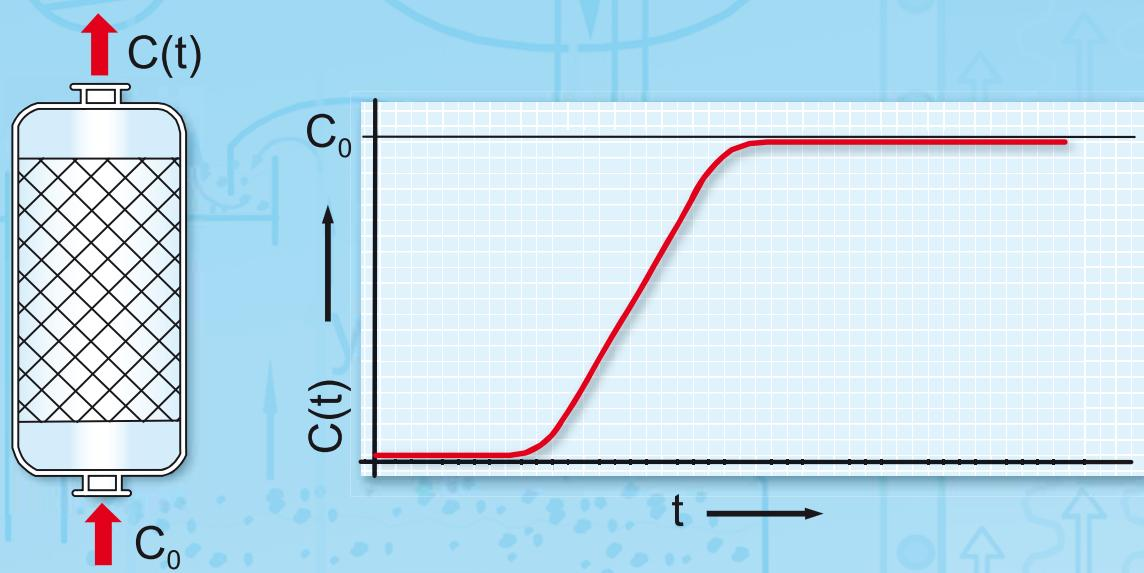
*Idealised breakthrough curve for a packed bed adsorber:*
