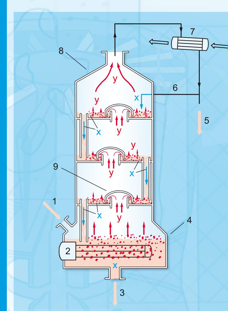
Simplified illustration of a rectification column:
