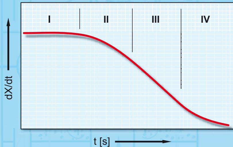
Drying characteristics of a solid with division into drying sections (I-IV):
