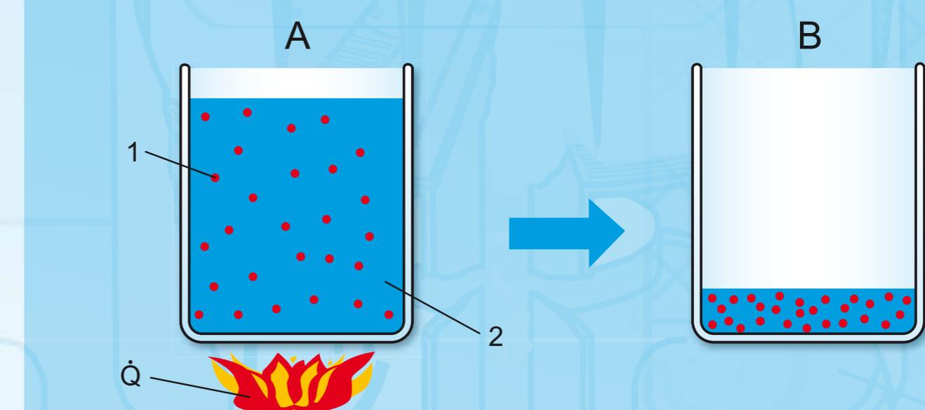
Principle of increasing the concentration of a solution by evaporating the solvent:
