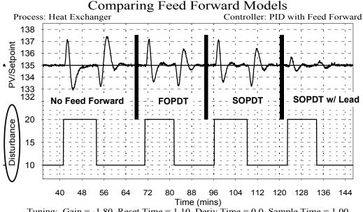
Tuning: Gain = -1.80, Reset Time = 1.10, Deriv Time = 0.0, Sample Time = 1.00 Process Model: Gain(Kp) = -0.39, T1 = 0.96, T2 = 0.0, TD = 0.80, TL = 0.0 Disturbance Model: Gain(Kd) = -0.146, T1 = 0.735, T2 = 0.735, TD = 0.822, TL = -3.41
