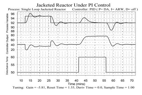
Set point tracking and disturbance rejection performance of the Jacketed Reactor process
