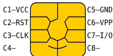
Gambar 9 Smart Card's pin contact
