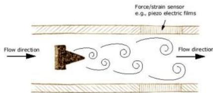
Gambar 4. Prinsip Kerja Vortex Flowmeter.
