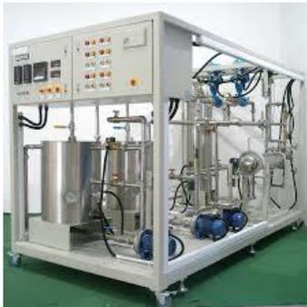
Gambar 1. Alat Boiler heating batching control trainer ( Model : Se 107)
