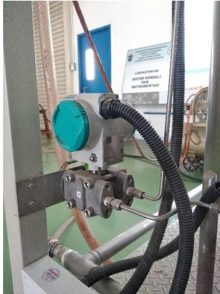
**Gambar 2.3 Differential Pressure Level Transmitter**
