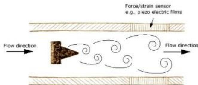
**Gambar 2.9 Prinsip Kerja Vortex Flowmeter.**
