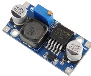
Gambar 2. 7 Buck Converter Modul LM2596
