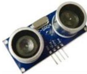
**Gambar 2.5** Sensor Ultrasonik HC SR-04
