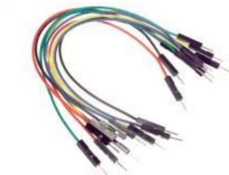
**Gambar 2.4** Kabel Jumper
